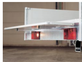
Pullout beams at backside
