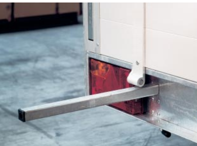
Pullout beam at backside
